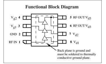
and flexibility. The CMM0333 is packaged in a low-cost, space efficient SO-8 power package that gives excellent electrical stability and thermal handling performance with a  $R_{\Theta}$  of less than 18° C/W. The part is designed to require minimal external circuitry for bias matching, simplifying design and keeping board space and cost to a minimum.
