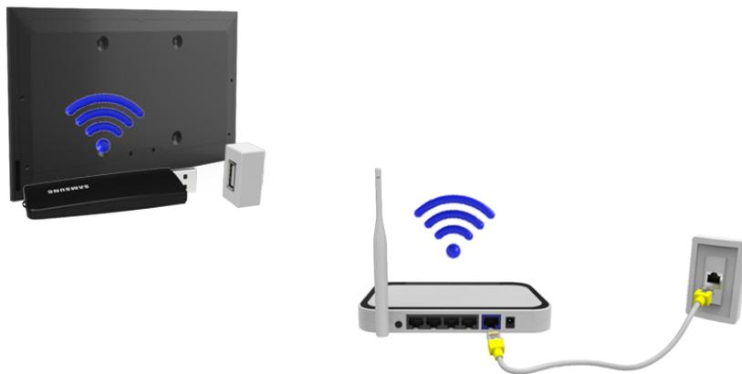
Using the wireless LAN adapter may cause image retention or radio interference on some TV channels. In those cases, use one of the following methods.
