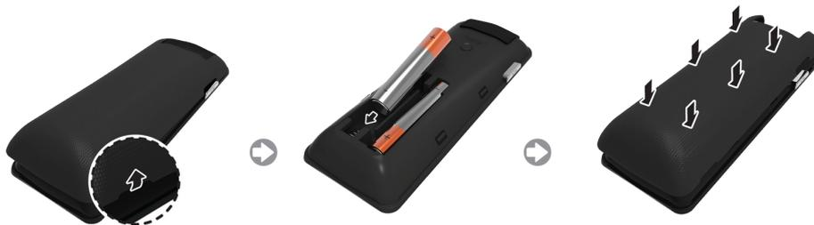
1. Slightly lift the battery cover by pulling the strap or using a plastic card. Next, pull on the cover's notch with a fingernail to remove the cover completely.
