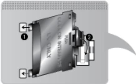
1. Insert the CI CARD Adapter into the two holes on the product 1.
