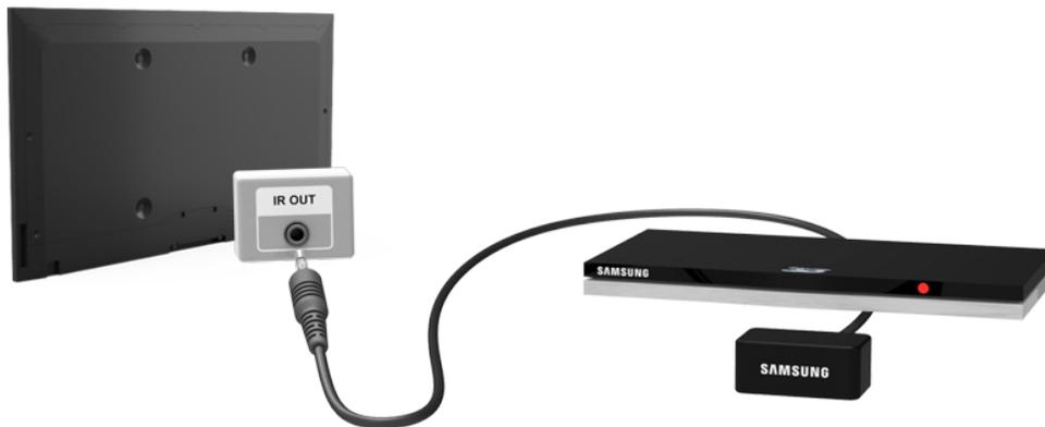
Keep a distance of 5 cm at least between the IR EXTENDER CABLE and the external device, as the illustration shows. Face the IR EXTENDER CABLE toward the external device's remote control signal receiver. Note that it should be no obstacle between IR Extender and external device. The presence of an obstacle will interfere with the transmission of the remote control signal.
