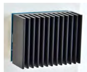
Vertical test position of TE-CORE /RF with heat sink Sk422-33
