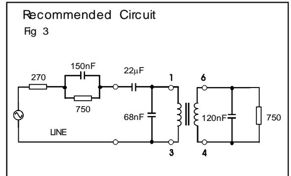
In practice, the 750Ω load resistor will connect to a low output impedance TX driver. The 120nF capacitor, which should have a temperature stable dielectric, should appear in parallel with the 750Ω resistor (rather than in parallel with the transformer winding) to obtain flat TX response to line.
