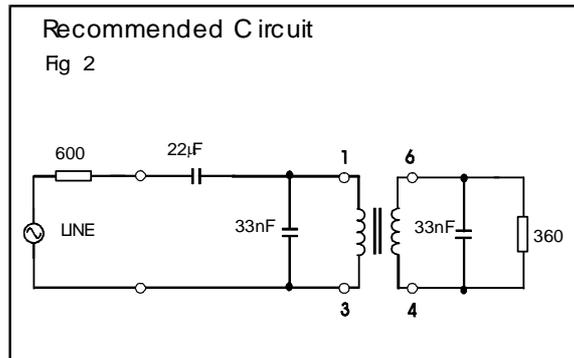
In practice the 360Ω load resistor in figure 2 will connect to a low output impedance TX driver. The 33nF capacitor on the load side should appear in parallel with the 360Ω resistor (rather than in parallel with the transformer winding) to obtain flat TX response to line.
