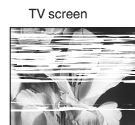
TV screen Playback picture containing noise bars
