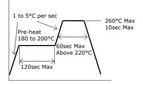
• Recommended Hand Soldering Condition
