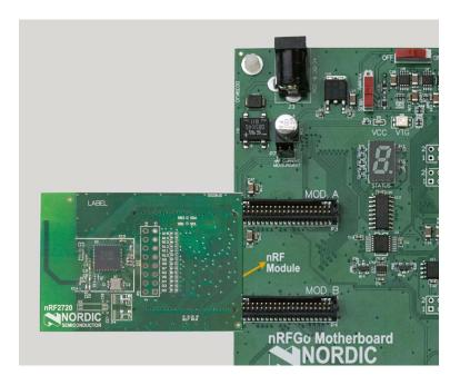
Figure 3. nRF module connectors
