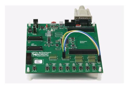
Figure 12. RS232 header P15 connected to IO header
