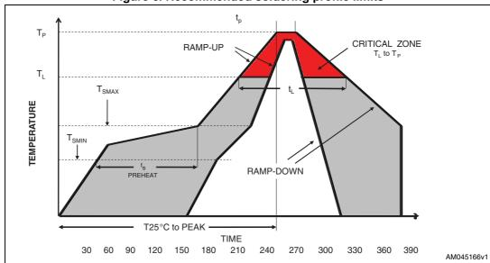
Figure 6. Recommended soldering profile limits
