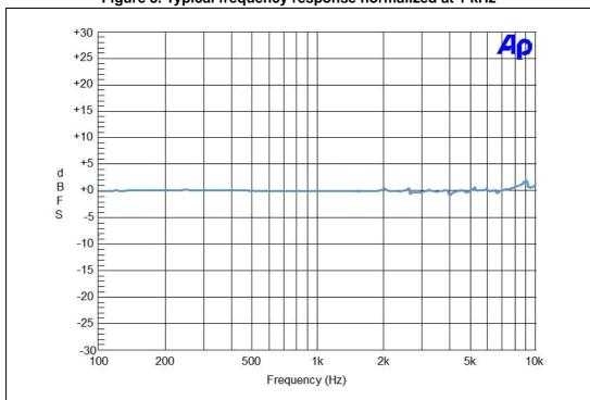
Figure 3. Typical frequency response normalized at 1 kHz
