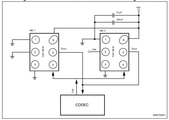
Power supply decoupling capacitors (100 nF ceramic, 10 µF ceramic) should be placed as near as possible to pin 6 of the device (common design practice).
