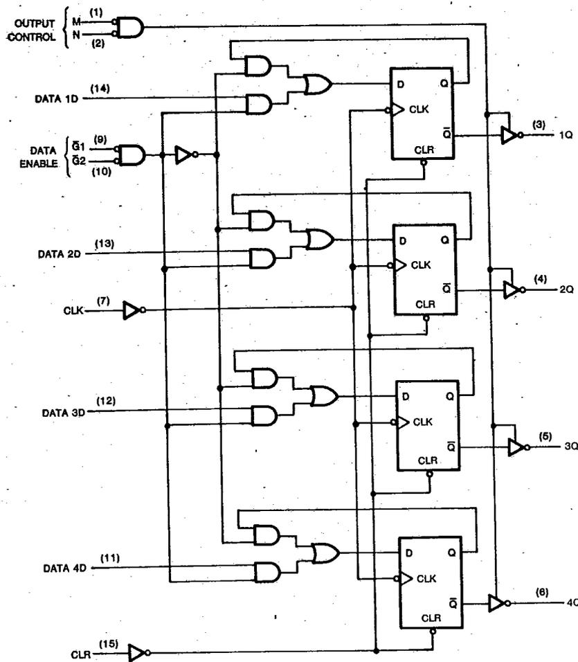
**KS54AHCT 173 4-Bit D-Type Registers with 3-State Outputs**
