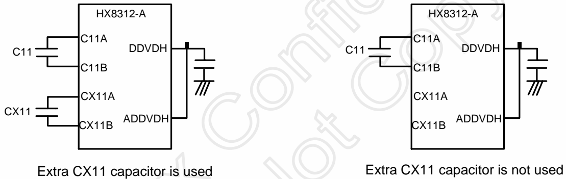
Figure 13. 2 Configuration of the Step up Circuit 1
