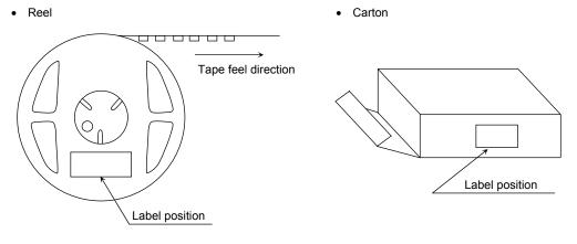
The aluminum package in which the reel is supplied also has the label attached to center of one side.
