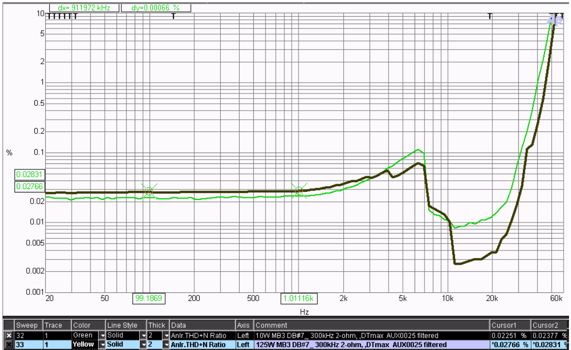
Figure 4 THD+N vs. Frequency at 10W and 125W
