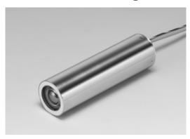
The H9319 series photon counting heads are designed to perform photon counting by just connecting to a PC. The H9319 series includes a 25-mm (1") diameter head-on photomultiplier tube, a photon counting circuit, a high-voltage power supply circuit, counter and a microprocessor. Data transfer, measurement time and other necessary adjustments can be controlled by commands from the PC through the RS-232C interface.
