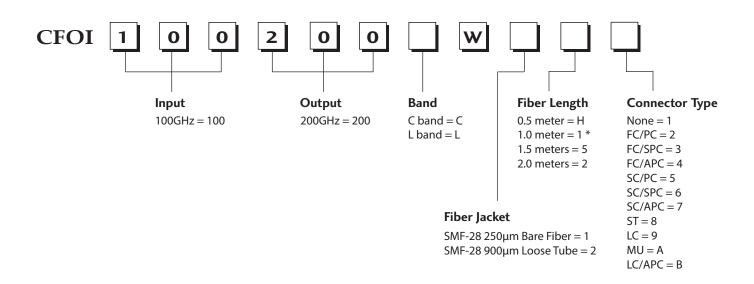
\* The tolerance of fiber length is +/-0.1m. 1 meter is standard. The lead-time for special fiber length will be longer.
