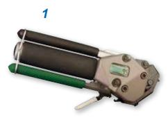
The 601-108 Nano Band-Master™ ATS Tool weighs 1.18 lbs., and is designed for nano flat .075" width clamping bands (601-500, 601-504 and 601-508) in a tension range from 20 to 50 lbs. Calibrate at 50 lbs. ± 3 lbs. for most shield terminations. Tool and band should never be lubricated.
