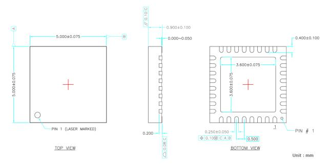
Figure 10.1 VQFN-32 Package Dimensions
