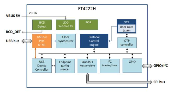
Figure 2.1 FT4222H Block Diagram
