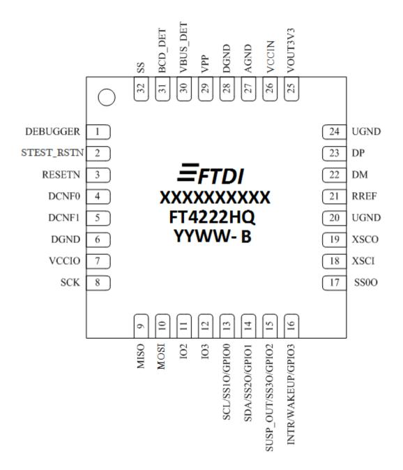
Figure 3.1 Pin Configuration VQFN-32 (top-down view)
