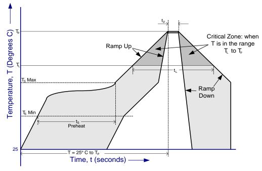
Figure 10.3 FT4222H Solder Reflow Profile
