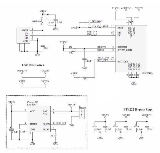
Figure 7.5 USB Battery Charging Detection
