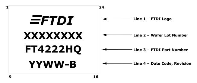
Figure 10.2 VQFN-32 Package Markings
