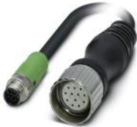
Sensor/Actuator cable, 12-position, PUR/PVC, Black RAL 9005, shielded, Plug straight M12-SPEEDCON, A-coded, on Socket straight M23, Cable length: 0.5 m
