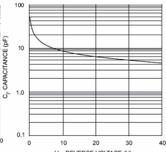
Fig. 2 Typ. Junction Capacitance vs Reverse Voltage
