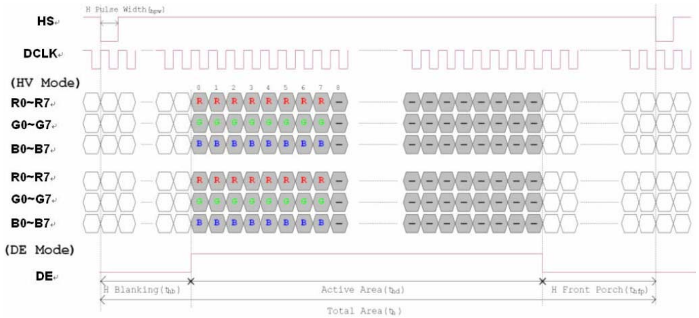
Figure 3.1 Horizontal input timing diagram
