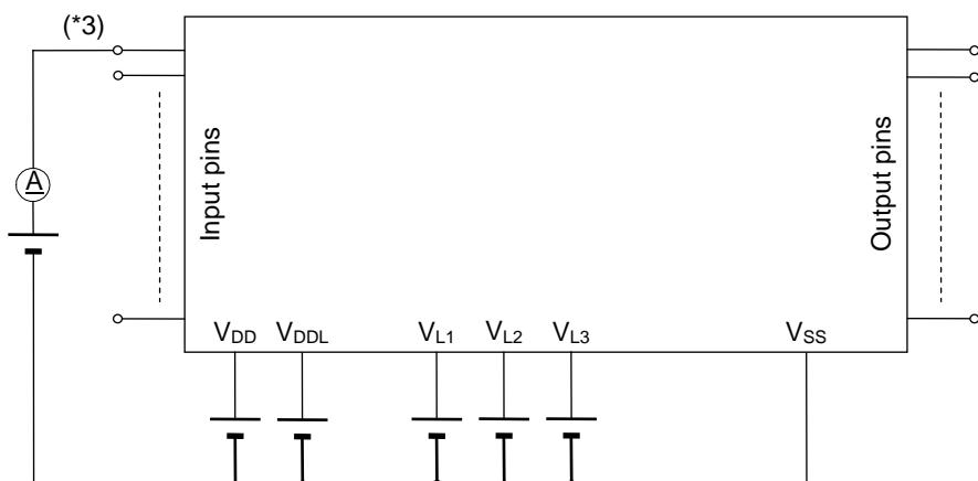
\*3: Measured at the specified output pins.
