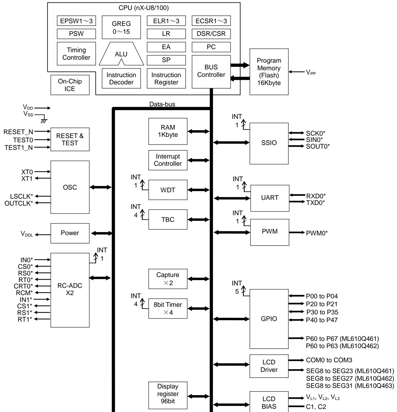
**Figure 1 ML610Q461/ML610Q462/ML610Q463 Block Diagram**
