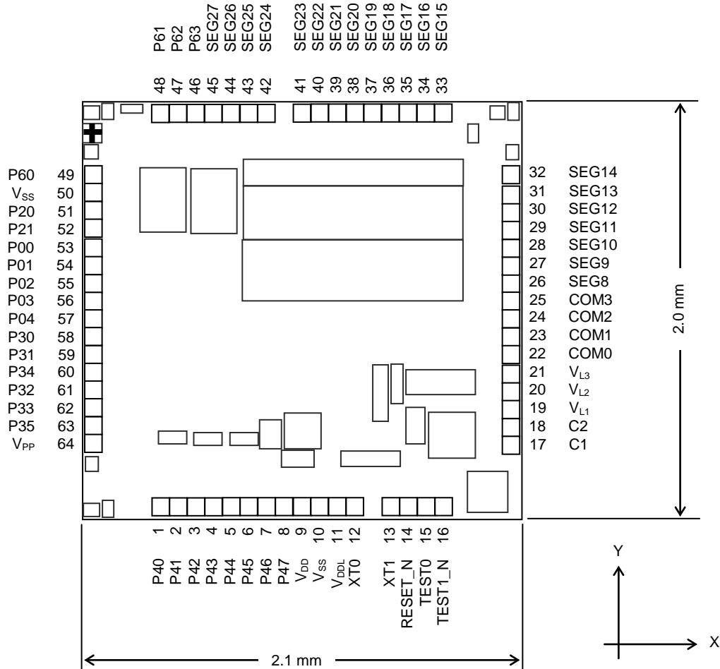
Note: The assignment of the pads P30 to P35 are not in order.
