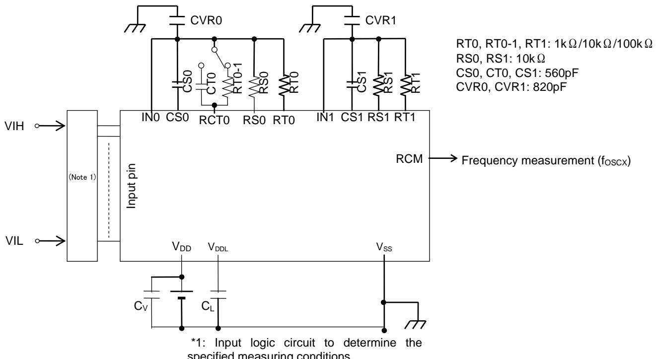
Condition for V<sub>DD</sub>=1.25 to 3.6V
