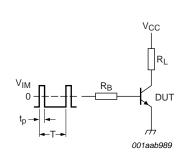
$V_{IM} = -6 \text{ to } + 8V; \, t_p = 20 \; \mu s; \\ \delta = \frac{t_p}{T} = 0.01$   $R_B$  and  $R_L$  calculated from  $I_{Con}$  and  $I_{Bon}$  requirements.
