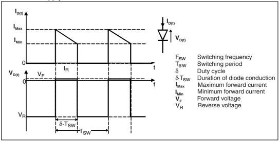
The reverse losses in a diode are the result of a reverse bias applied on the diode. They are due to the leakage current ( $I_R$ ). This parameter ( $I_R$ ) increases exponentially with the junction temperature. Most of time, the reverse losses are negligible for bipolar and silicon carbide diodes. For silicon Schottky structured diodes, these losses should be accurately estimated as they are the main origin of the thermal runaway risk phenomenon ( $See\ AN1542$ ).
