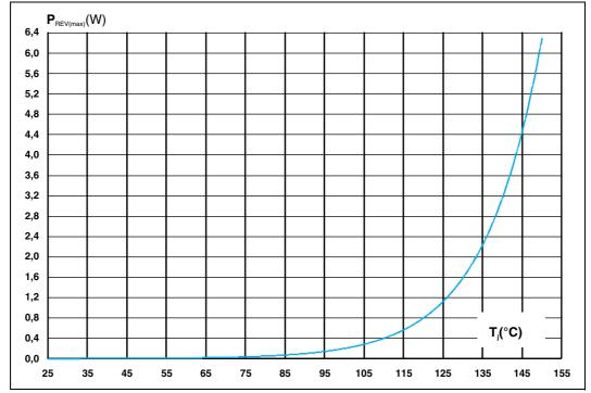
Figure 6. Maximum reverse losses versus the junction temperature
