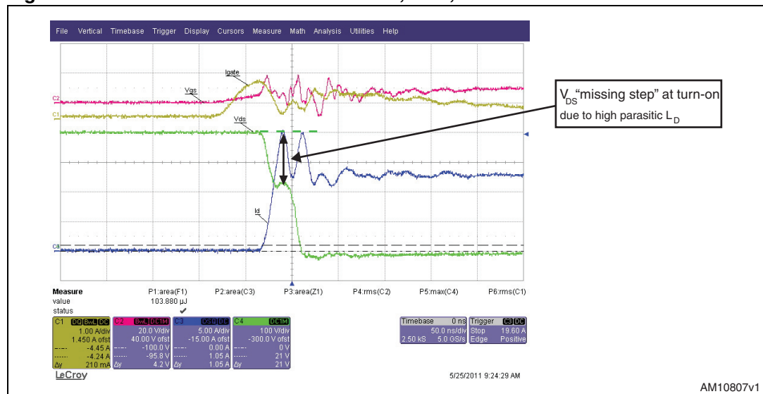
Figure 44. Turn-on of STW77N65M5@400 V, 13 A, 25 °C
