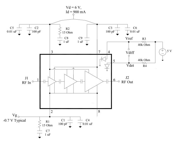
Vg can be biased from either side (bond pad 2 or bond pad 8), and the non-biased side can be left open. Vd must be biased from both sides (bond pad 3 and bond pad 7).
