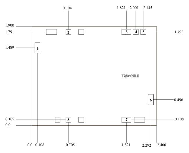
Unit: millimeters Thickness: 0.10
