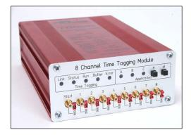
The **Time Tagging Module TTM8000** is an 8 channel time-to-digital converter. Incoming signals are tagged with a 64 bit timestamp. The time resolution (bin size) depends on the selected measurement mode (between 82.3 and 1ps).
