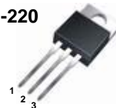
1.Gate 2. Drain 3. Source
