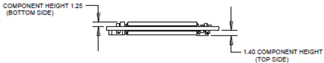
Figure 4-4 : mSATA 8-64GB Side View
