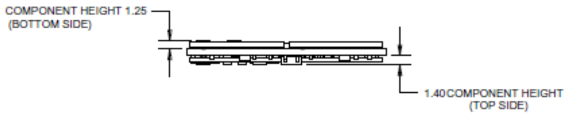
Figure 4-6 : mSATA 128-256GB Side View
