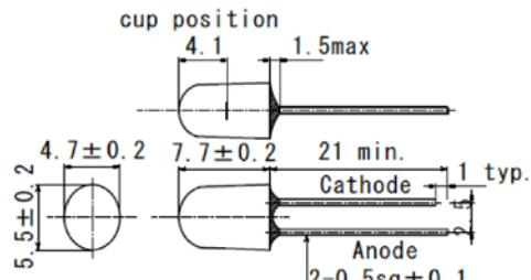
**Figure-8 Ø 5Mold (Type 46)**
