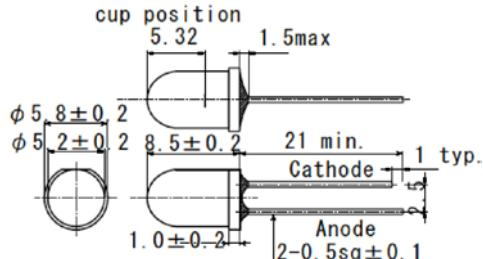
**Figure-3 Ø 5Mold (Type 03)**
