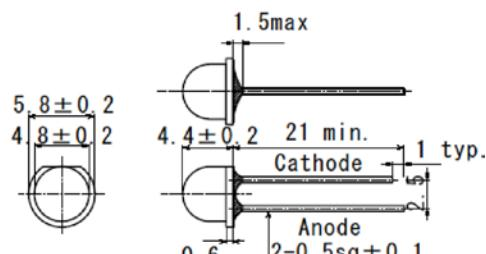
**Figure-9 Ø 4Mold (Type 41)**
