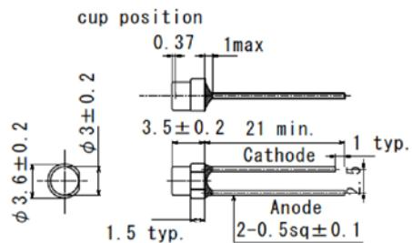
**Figure-12 Ø 3Mold (Type 33)**
