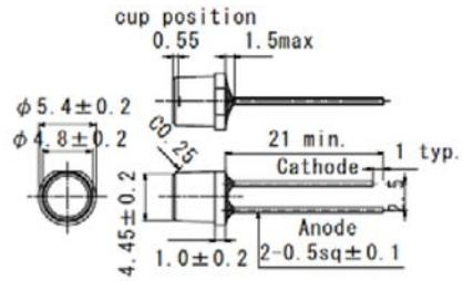
**Figure-6 Ø 5Mold (Type 06)**
