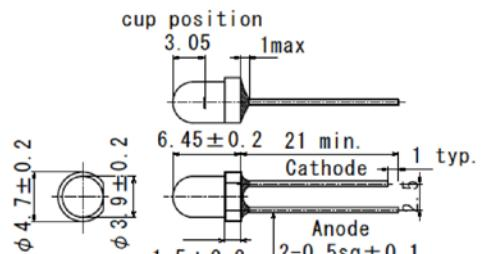
**Figure-10 Ø 4Mold (Type 42)**
