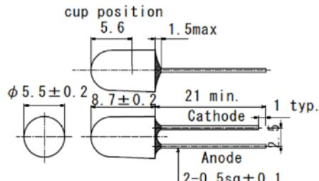
**Figure-7 Ø 5Mold (Type 09)**
