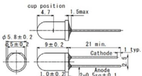
**Figure-2 Ø 5Mold (Type 02)**
