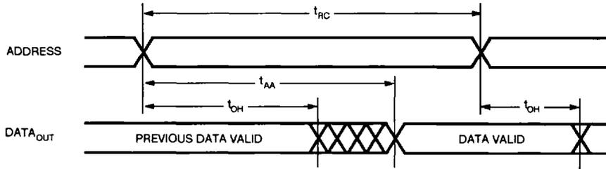
**TIMING WAVEFORM OF READ CYCLE NO. 3<sup>(1, 3, 4)</sup>**
