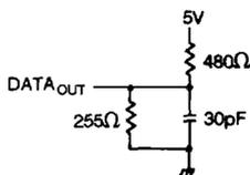
Figure 1. Output Load
