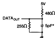
Figure 2. Output Load
