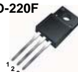
1.Gate 2. Drain 3. Source
