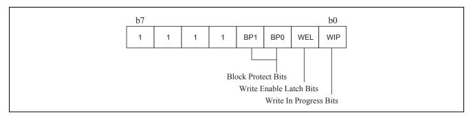
WIP bit: The Write In Progress (WIP) bit indicates whether the memory is busy with a Write or Write Status Register cycle.
