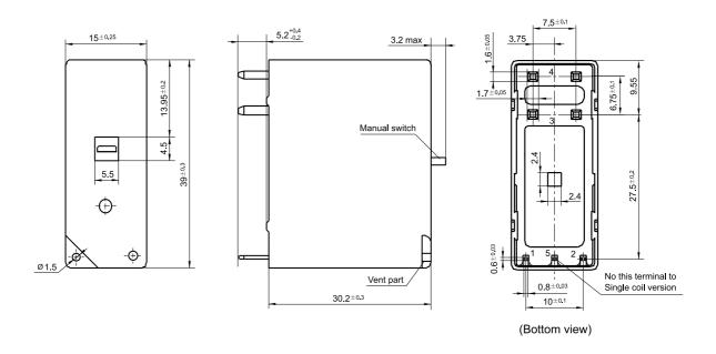
Remark: In case of no tolerance shown in outline dimension: outline dimension ≤1mm, tolerance should be ±0.2mm; outline dimension >1mm and ≤5mm, tolerance should be ±0.3mm; outline dimension >5mm, tolerance should be ±0.4mm.
