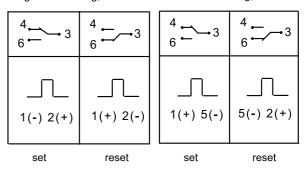
Single coil latching, 1 Form B Double coils latching, 1 FormB
