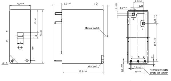
Remark: When the manual switch is pitched on point a, the contact is open; when the manual switch is pitched on point b, the contact is closed.
