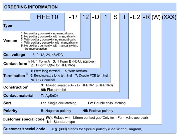
Notes: 1) H means that relay is on the "reset" status when delivery; D means that relay is on the "set" status when delivery.
