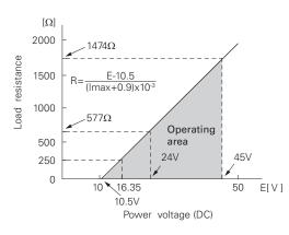
Note: For communication with HHC  $^{(1)}$  (Model: FXW), min. of 250  $\Omega$  required.
