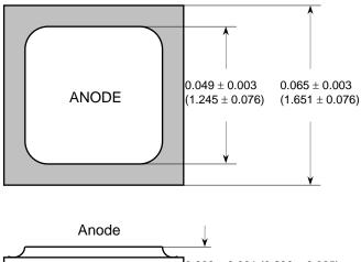
Top side metalization - Aluminum - 25 kÅ minimum. Bottom side metalization - Ti/Ni/Ag - 30 kÅ minimum
