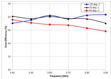
T1G6003028-FL PAE vs. Temp. V<sub>DS</sub> = 28 V, I<sub>DQ</sub> = 200 mA; Pulse: 100 μs, 20%
