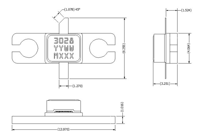
This package is lead-free/RoHS-compliant. The plating material on the leads is NiAu. It is compatible with both lead-free (maximum 260 °C reflow temperature) and tin-lead (maximum 245 °C reflow temperature) soldering processes.
