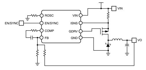
Figure 1. NCV8852 Application Diagram
