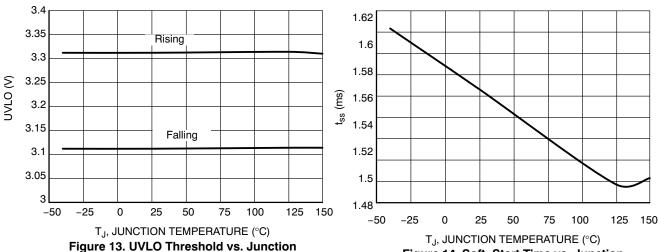
Figure 13. UVLO Threshold vs. Junction Temperature
