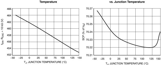
Figure 7. Switching Frequency ( $R_{OSC}$  = 10 k $\Omega$ ) vs. Junction Temperature
