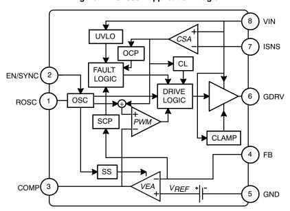
Figure 2. NCV8852 Simple Block Diagram
