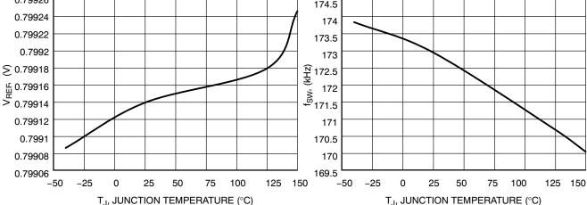
Figure 5. Reference Voltage vs. Junction
