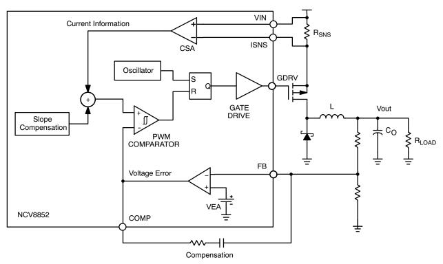
Figure 15. Current Mode Control Schematic
