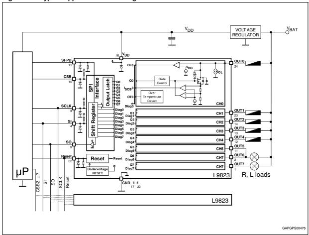
For higher current driving capability more outputs of the same kind can be paralleled. In this case the maximum flyback energy should not exceed the limit value for single output.
