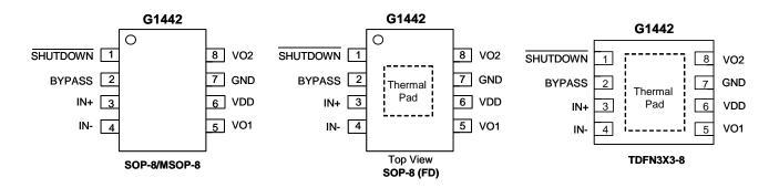
Note: Recommend connecting the Thermal Pad to the GND for excellent power dissipation.
