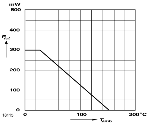
Figure 2. Admissible Power Dissipation vs. Ambient Temperature
