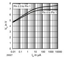
Figure 5. Typical Reverse Voltage  $V_{\text{R}}$  vs. Reverse Current  $I_{\text{R}}$
