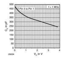
Figure 2. Typical Capacitance  $\mathrm{C}_{\mathrm{D}}$  vs. Reverse Voltage  $\mathrm{V}_{\mathrm{R}}$
