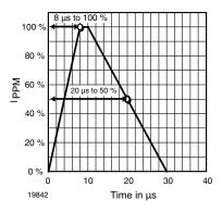
Figure 1. 8/20 µs Peak Pulse Current wave form acc. IEC 61000-4-5
