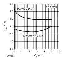
Figure 3. Typical Capacitance C<sub>D</sub> vs. Reverse Voltage V<sub>R</sub>
