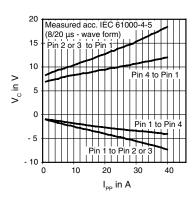
Figure 6. Typical Clamping Voltage vs. Peak Pulse Current IPP
