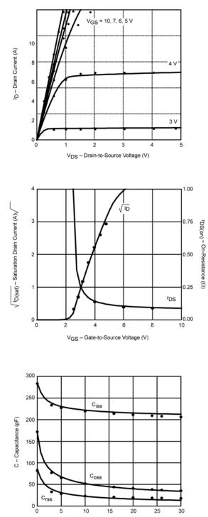
V<sub>DS</sub> – Drain-to-Source Voltage (V)
