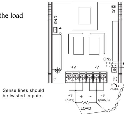
Sense lines should be twisted in pairs
