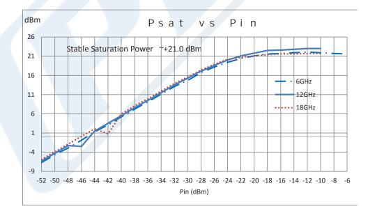
40 dB Gain, 19 dBm, 6 GHz to 18 GHz, Limiting Amplifer, -20 to 20 dBm Pin, SMA from Pasternack Enterprises has same day shipment for domestic and International orders. Our RF, microwave and millimeter wave products maintain a 99% availability and
