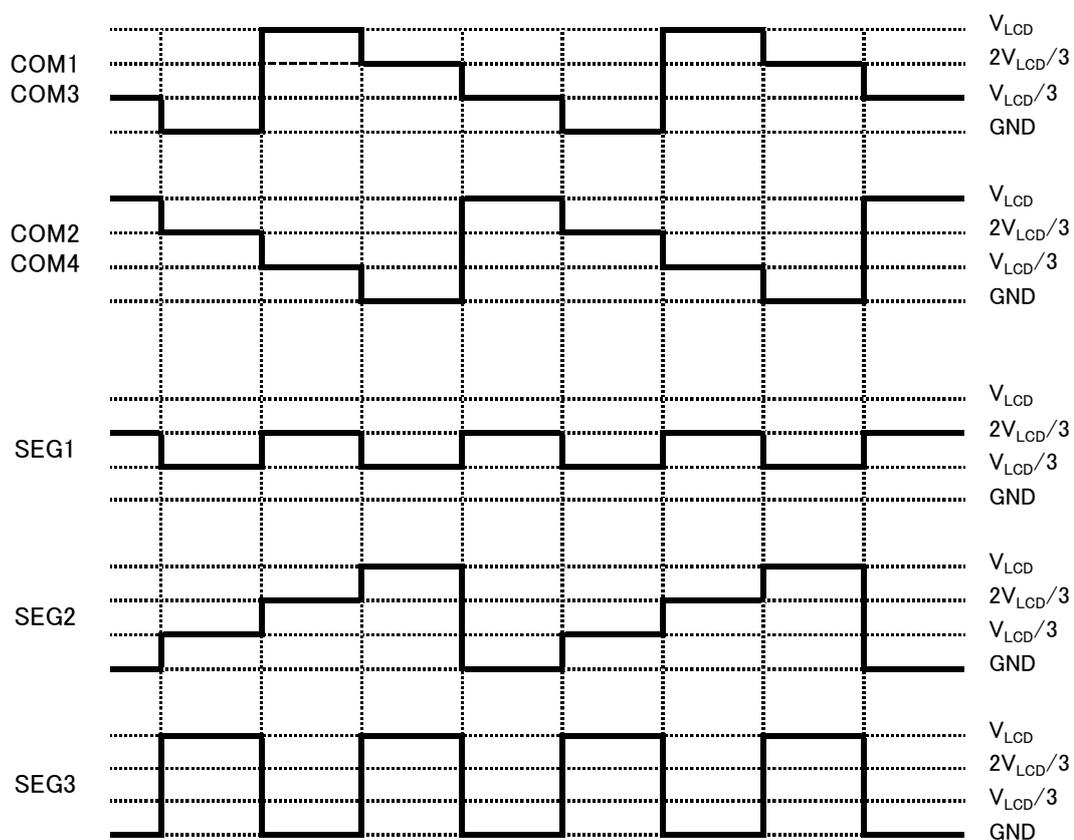
● Common and segment output waveforms
