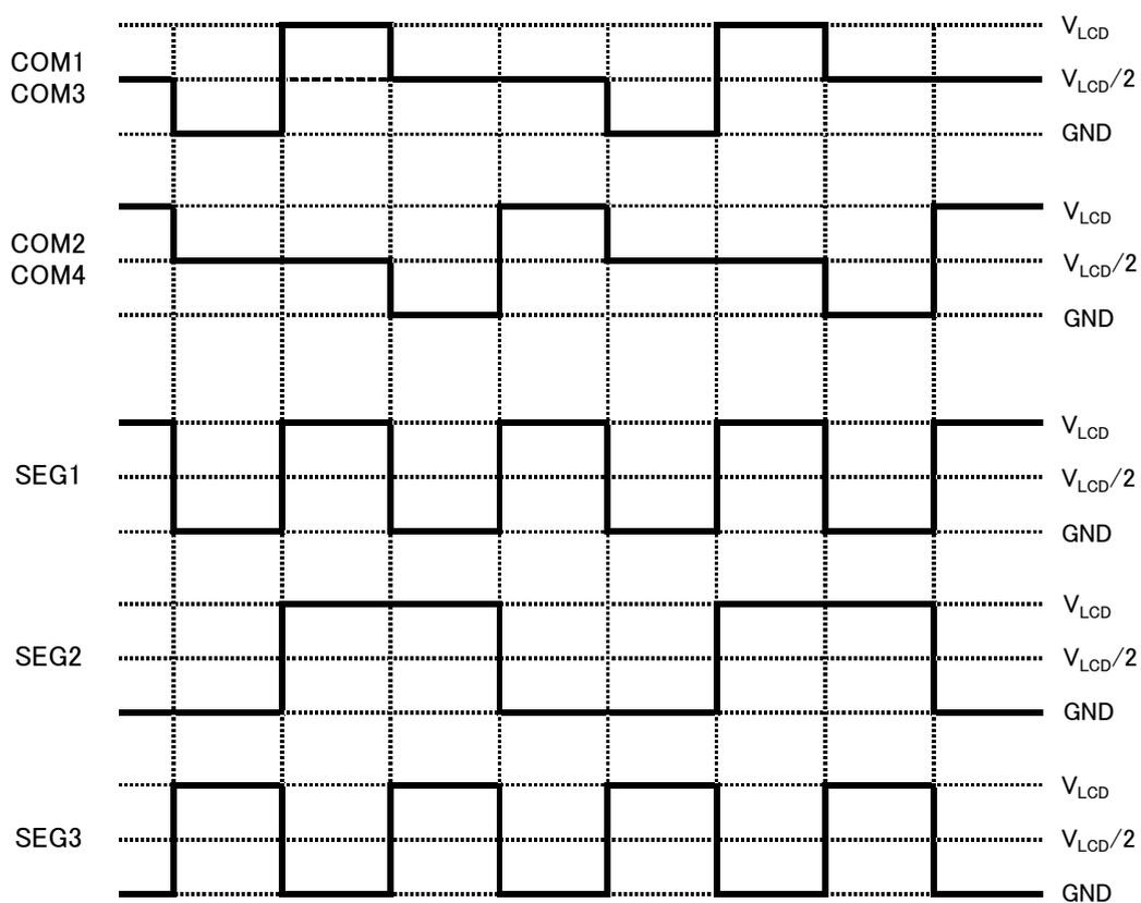
● Common segment output waveform
