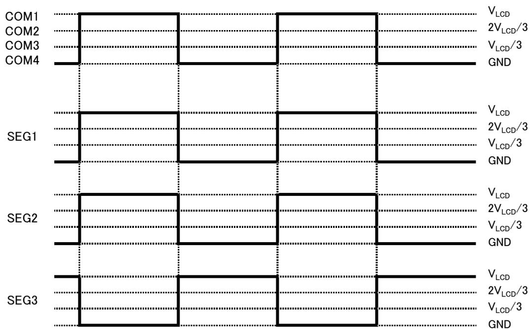
● Common and segment output waveforms
