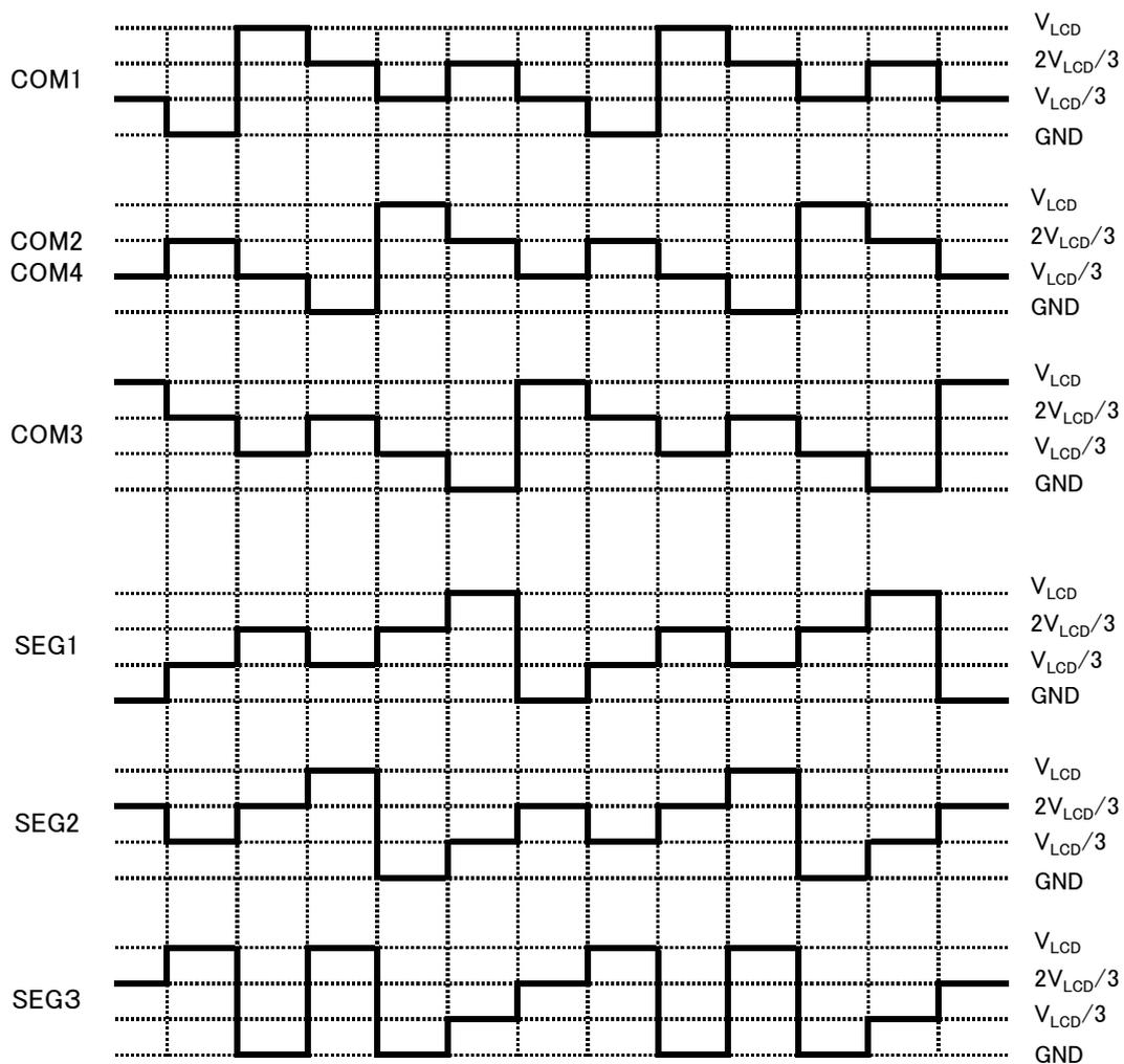
● Common and segment output waveforms
