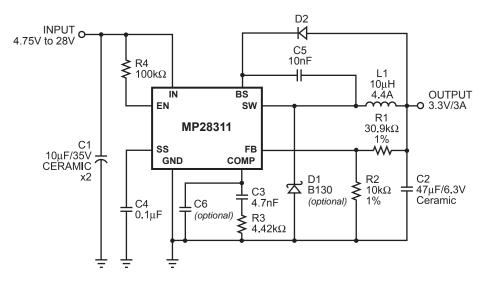
Figure 4—MP28311 with 3.3V Output, 47µF/6.3V Ceramic Output Capacitor
