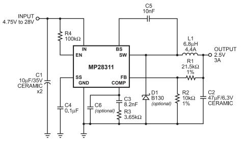
Figure 3—MP28311 with 2.5V Output, 47µF/6.3V Ceramic Output Capacitor
