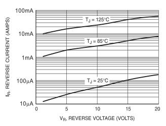
Figure 3. Typical Reverse Current
