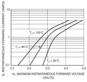
Figure 2. Maximum Forward Voltage
