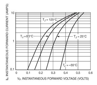
Figure 1. Typical Forward Voltage
