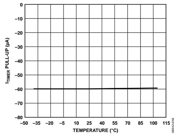
Figure 16. I<sub>TIMER</sub> Pull-Up vs. Temperature
