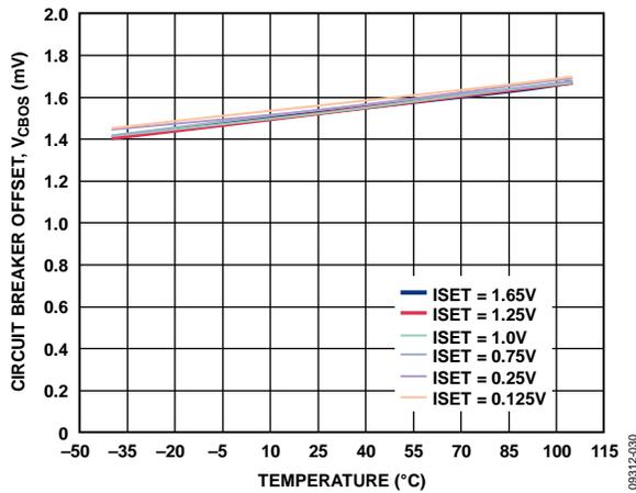
Figure 30. Circuit Breaker Offset vs. Temperature, ADM1075-2
