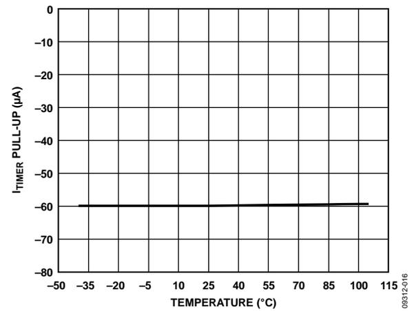
Figure 16. I<sub>TIMER</sub> Pull-Up vs. Temperature
