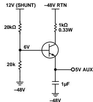
Figure 55. Powering *iCoupler* from -48 V Supply
