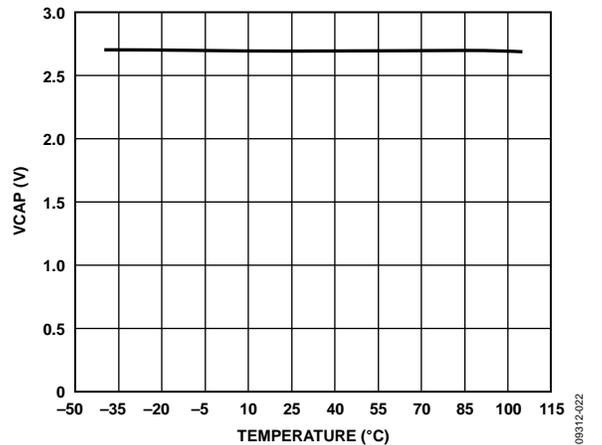
Figure 22. VCAP vs. Temperature (I<sub>VCAP</sub> = 100 µA)
