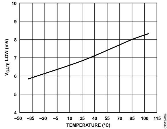
Figure 9. V<sub>GATE LOW</sub> vs. Temperature (I<sub>GATE</sub> = 100 μA)
