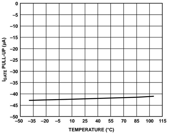
Figure 13. I<sub>GATE</sub> Pull-Up vs. Temperature
