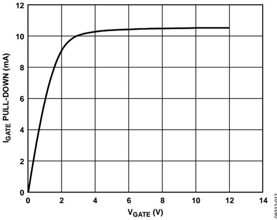
Figure 12. I<sub>GATE</sub> Pull-Down vs. V<sub>GATE</sub>
