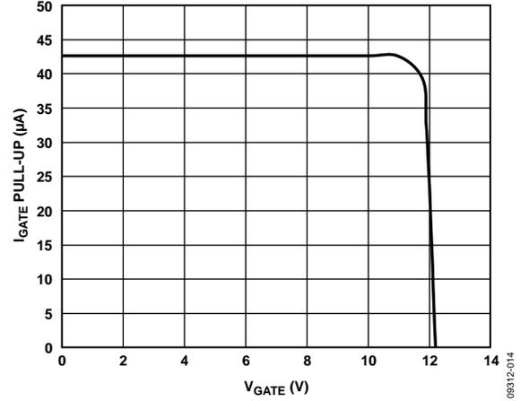
Figure 14. I<sub>GATE</sub> Pull-Up vs. V<sub>GATE</sub>
