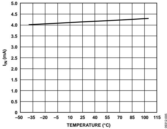
Figure 5. I<sub>IN</sub> vs. Temperature
