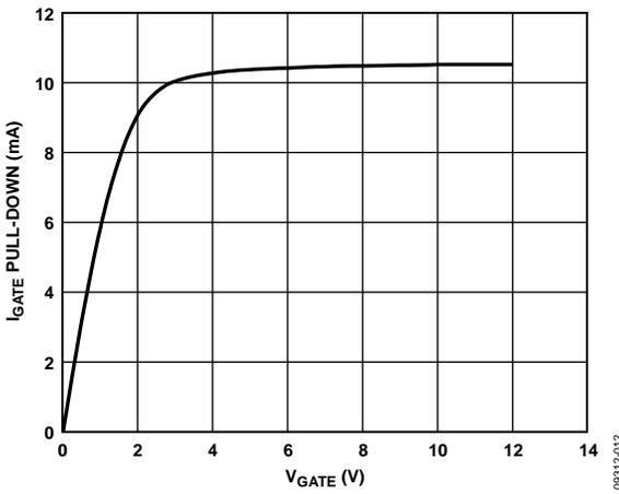
Figure 12. I<sub>GATE</sub> Pull-Down vs. V<sub>GATE</sub>
