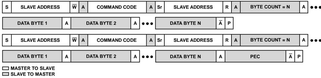
Figure 62. Block Read and Block Read with PEC
