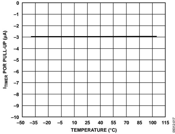
Figure 17. I<sub>TIMER</sub> POR Pull-Up vs. Temperature
