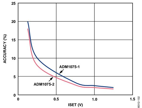
Figure 33. Worst-Case Hot Swap  $V_{SENSE}$  Accuracy vs.  $ISET$
