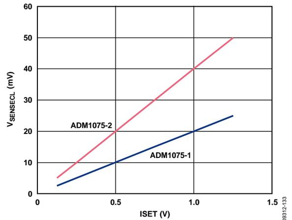
Figure 34. Typical Hot Swap  $V_{SENSECL}$  vs.  $ISET$
