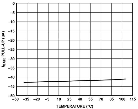
Figure 13. I<sub>GATE</sub> Pull-Up vs. Temperature
