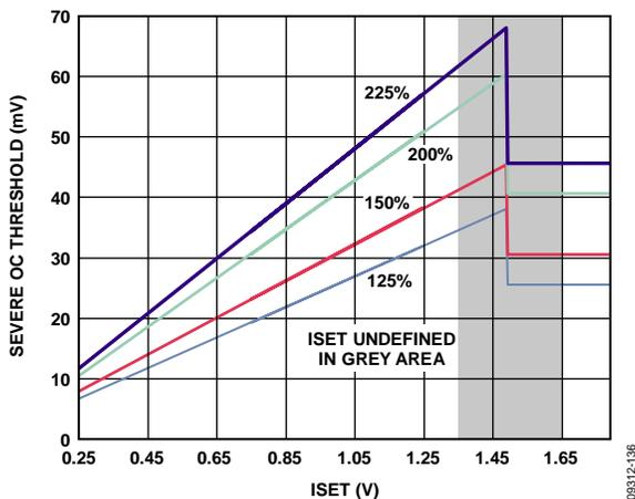
Figure 37. Severe OC Threshold vs. ISET, ADM1075-1
