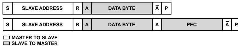
Figure 57. Receive Byte and Receive Byte with PEC
