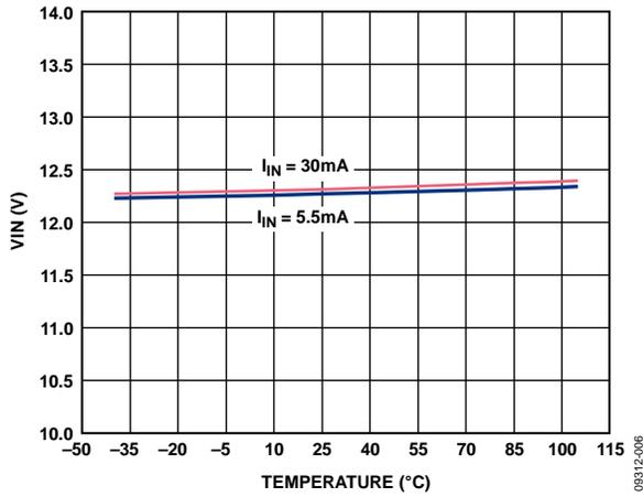
Figure 6. V<sub>IN</sub> vs. Temperature
