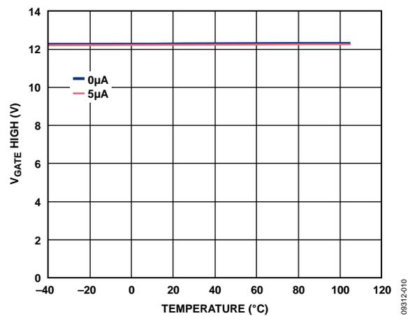
Figure 10. V<sub>GATE High</sub> vs. Temperature
