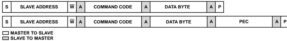
Figure 58. Write Byte and Write Byte with PEC
