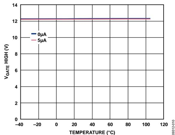
Figure 10. V<sub>GATE High</sub> vs. Temperature
