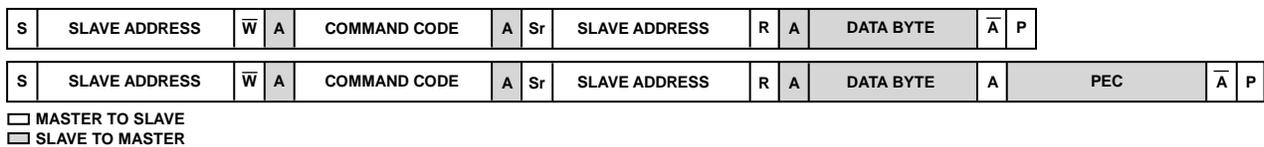
Figure 59. Read Byte and Read Byte with PEC
