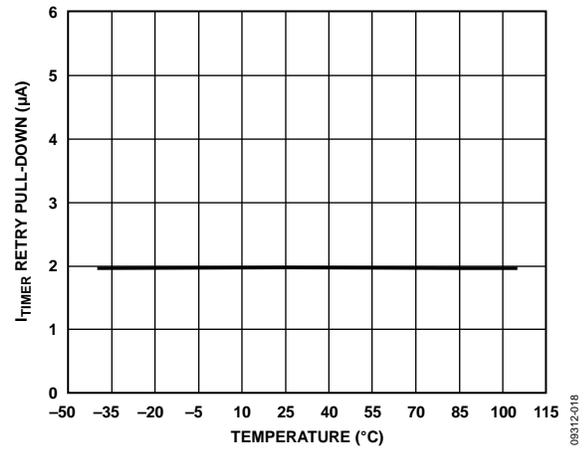
Figure 18. I<sub>TIMER</sub> Retry Pull-Down vs. Temperature
