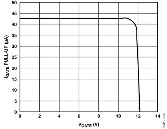
Figure 14. I<sub>GATE</sub> Pull-Up vs. V<sub>GATE</sub>
