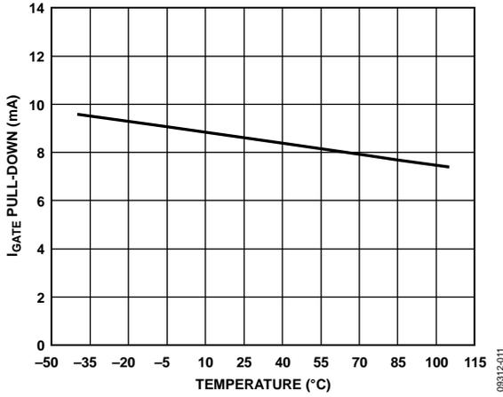
Figure 11. I<sub>GATE</sub> Pull-Down vs. Temperature
