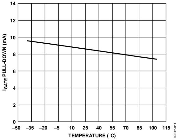
Figure 11. I<sub>GATE</sub> Pull-Down vs. Temperature
