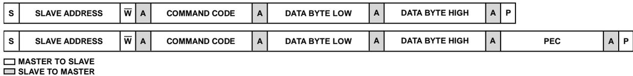
Figure 60. Write Word and Write Word with PEC
