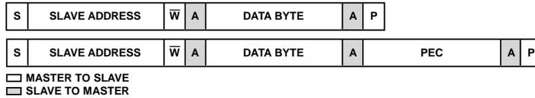
Figure 56. Send Byte and Send Byte with PEC
