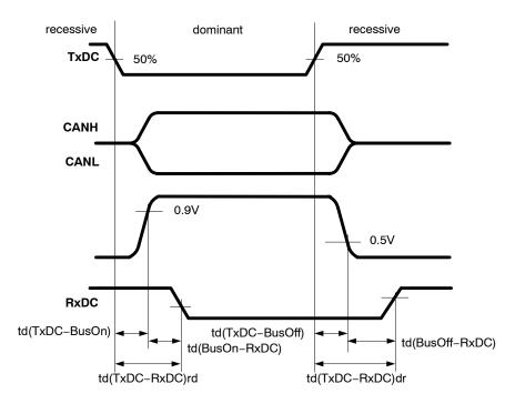
Figure 10. CAN Dynamic Characteristics
