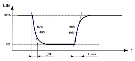
Figure 7. LIN Dynamic Characteristics – Transmitter Slope
