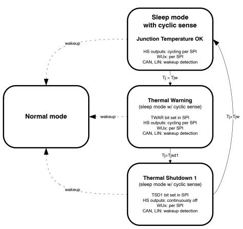
Figure 16. Thermal Protection in Sleep Mode
