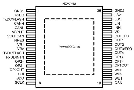
Figure 2. Package Pin-out
