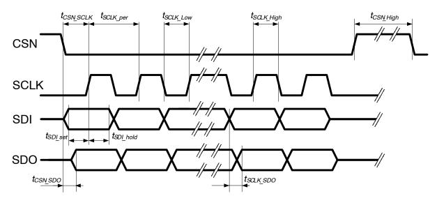
Figure 5. SPI Timing Parameters
