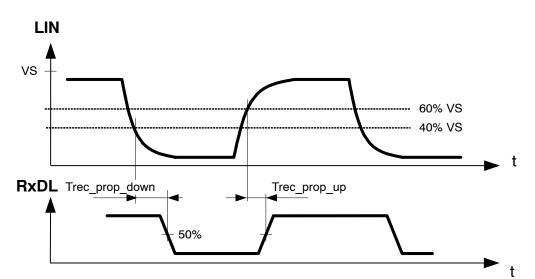
Figure 8. LIN Dynamic Characteristics – Receiver
