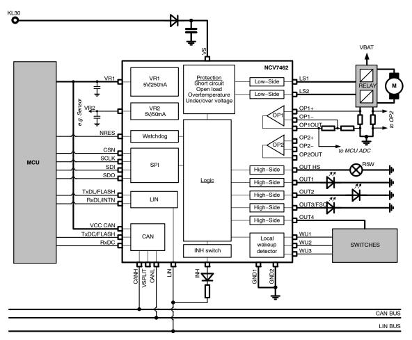
Figure 3. Application Diagram
