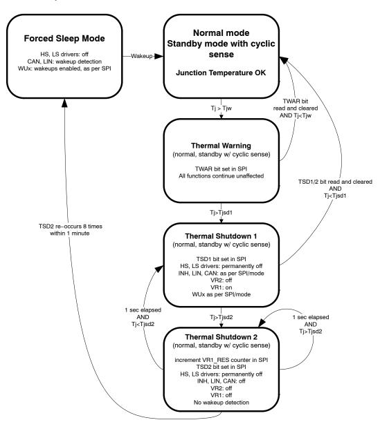
Figure 15. Thermal Protection in Normal and Standby Modes
