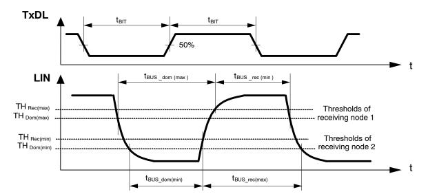
Figure 6. LIN Dynamic Characteristics – Duty Cycles
