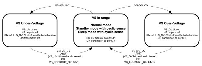
Figure 17. Under- and Over-voltage on VS Supply
