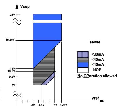
The operating range, and the corresponding maximum Isense, is defined by the Vsup-Vref range as shown in the graph.
