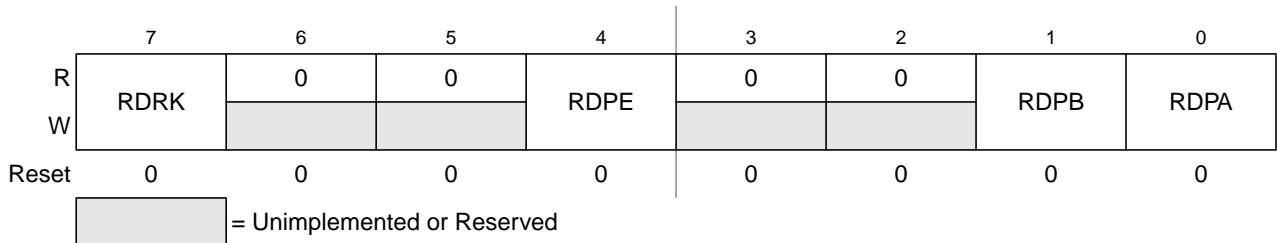
Figure 4-15. Reduced Drive Register (RDRIV)
